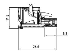
Contact Clip: Phbz, Tin Plated Wire Retention Spring: Stainless Steel Insulating Body: Polyamide, UL94V-0 Electrical Voltage Rating: 300 VAC Current rating: 10 AMPS 1500 VAC, Test time 60 sec Withstand Voltage: Wire Range: 12-26 AWG Mechanical -40°C to +105°C Operating Temperature: -40°F to +221°F Soldering Temperature: 260°C, 500°F for 5 seconds c Mus Safety Approval:
